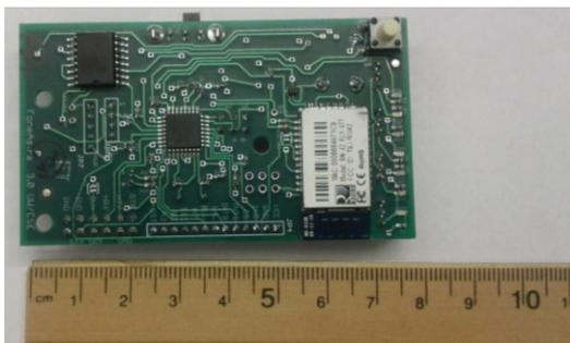
**Figure 2: FoneAstra, a reconfigurable interfacing board to enable wired or wireless communications between mobile devices and low-level sensors connected to the board.**
